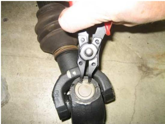
Using a pair of ring clip pliers, remove the two ring clips where the hub connects to the universal joint. Depending on when you last touched the universal joint, it may be easy to tap out the bearing cups or you may end up needing to press them out with a hydraulic press. I used a socket that was just slightly smaller than the cup diameter to tap out the universal joints. If they've been in there long enough to need a press, this may be a good opportunity to replace them with new ones.
