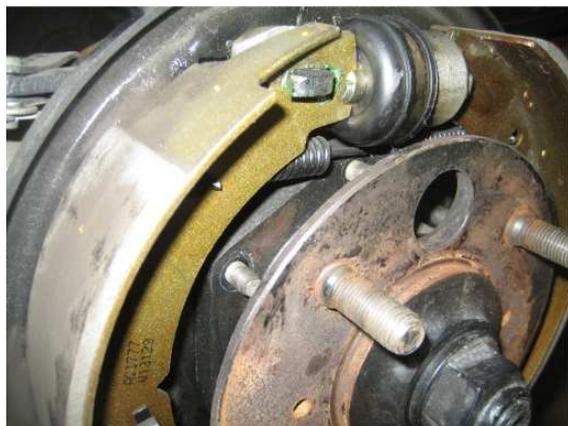
Next, pull the entire hub assembly out through the trailing arm. At this point you'll have the hub assembly with  $\frac{1}{2}$  the  $\frac{1}{2}$  shaft (I guess that makes it a quarter shaft).
